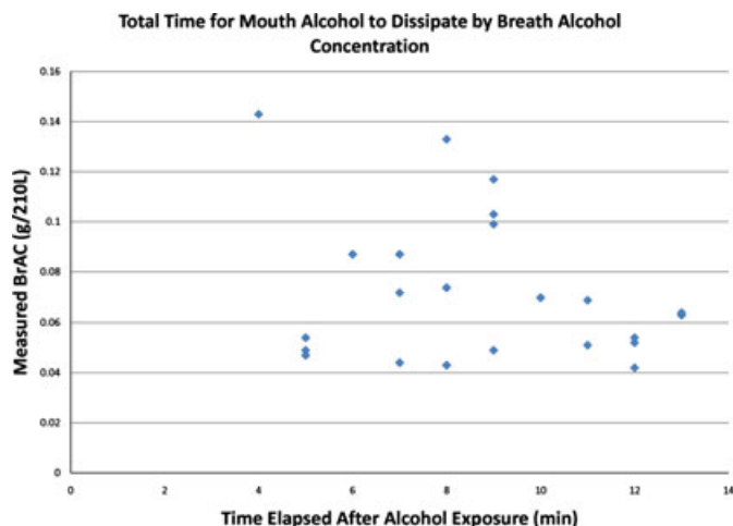
FIG. 2—Demonstrates that in this study, there is no relationship between the amount of time for mouth alcohol to dissipate and the unbiased breath alcohol concentration. The correlation coefficient was -0.263 ( SE = 0.028 , n = 23 ).
